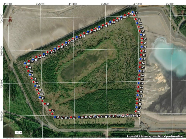
Passive seismic measurements on tailings embankment
